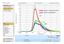
Setfos dipole emission and drift- diffusion model can be run directly from the Phelos control GUI.\*
