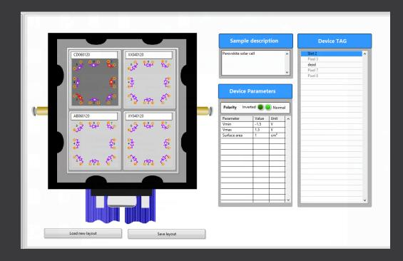
The Litos Lite software allows the user to easily switch between sample layouts and construct measurement routines e.g. JV stress cycle enabling data acquisition and analysis.
